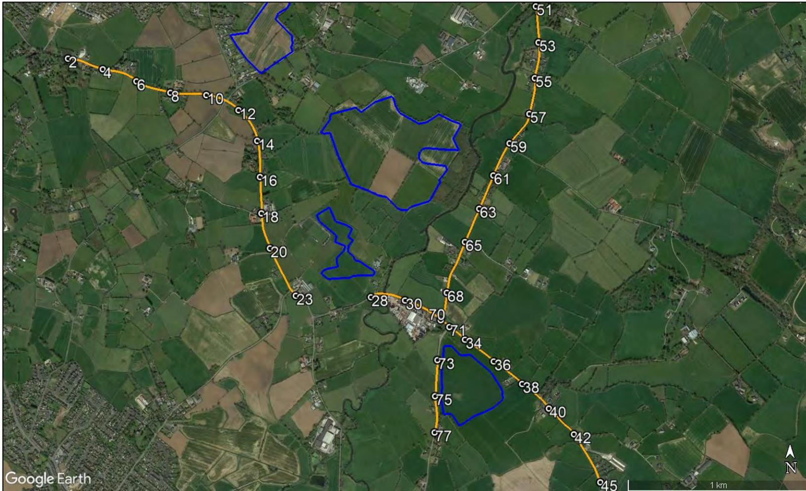
Figure 20 Sections of road towards which solar reflections are geometrically possible (orange) – aerial image
