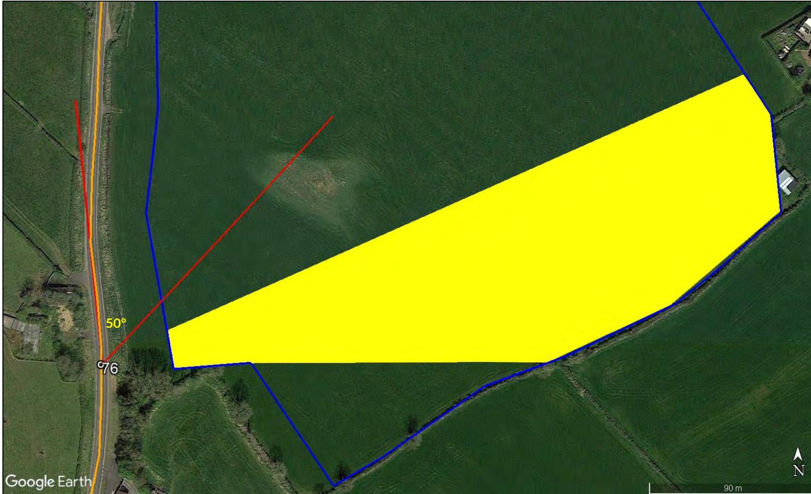
Figure 22 Reflecting area for road receptor 76 with respect to road user's primary field of view to the right side when travelling northbound
